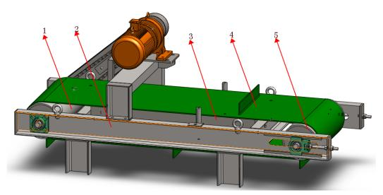
1. 头轮 head wheel 2.支架 machine frame 3.永磁磁芯 Permanent magnet magnetic core 4.皮带 belt 5.尾轮 foot wheel
