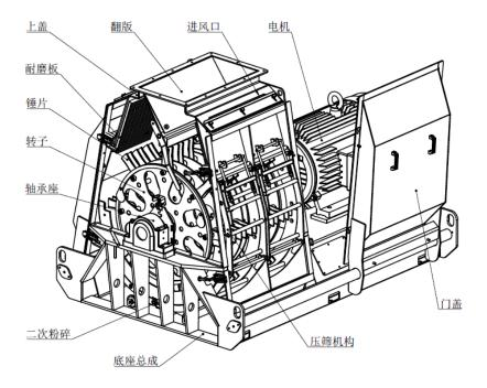
Base: the heavy-duty base is used to connect and support various parts of the grinder, reduce vibration, increase reliability, and extend life. The grinded materials are discharged from the discharge port at the lower part of the base.
