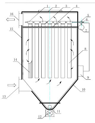
1 —Ejector nozzle 2 —upper cover 3 —Plug pipe 4 — tubesheet; 5 —Pulse valve 6 —Electromagnetic valve 7 —Air bag 8 —Filter bag 9 —Pulse controller 10 —Ash bucket 11 —; Screw conveyor 12 —discharger 13 —air inlet 14 —Filter bag framework; 15 —box of machine body 16—outlet
