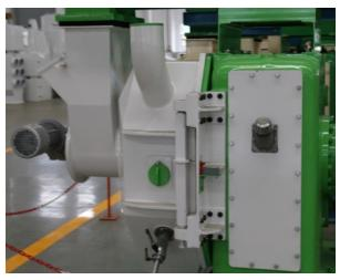
This machine is mainly composed of two parts: feeding system and main drive granulation system. The specific structure is shown in the system breakdown diagram as below:
